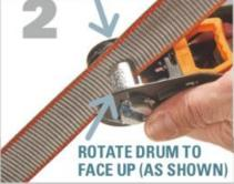
SLIDE THE WEBBING INTO THE PATENTED SLOTTED DRUM
